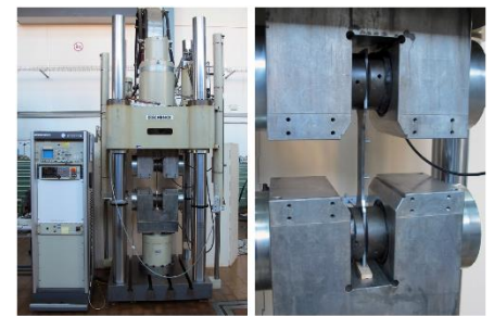
Test facility for fatigue tests
