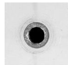
Shiny ring around the bore hole
