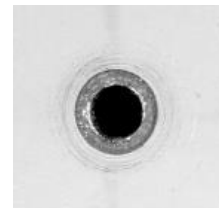
Shiny ring around the bore hole
