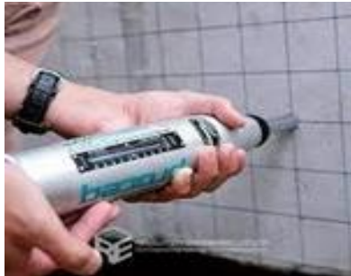
Schmidt hammer test
